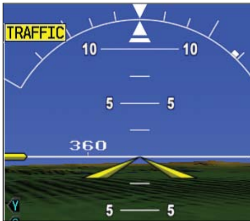
Figure 5-34 Pitch Scale with SVT Enabled
